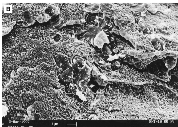
Fig. 9. Micrographs of PET/P2 70/30 w/w blends after tensile fracture: (A) ductile fracture; (B) fragile fracture.
