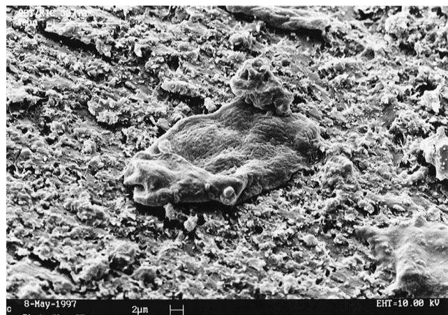
Fig. 7. Micrograph of the PET/ P2 30/70 w/w blend, showing a large island of PET in a matrix of P2 .
