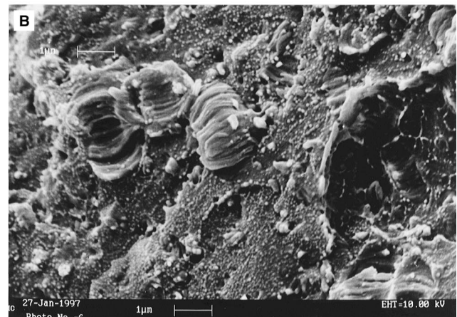
Fig. 6. Micrographs of: (A) PET/ P2 90/10 w/w blend, showing detail of the 'tree-ring' morphology of the droplet; (B) PET/ P2 60/40 w/w blend, showing that P2 droplets are always of the same dimensions, although more densely scattered.
